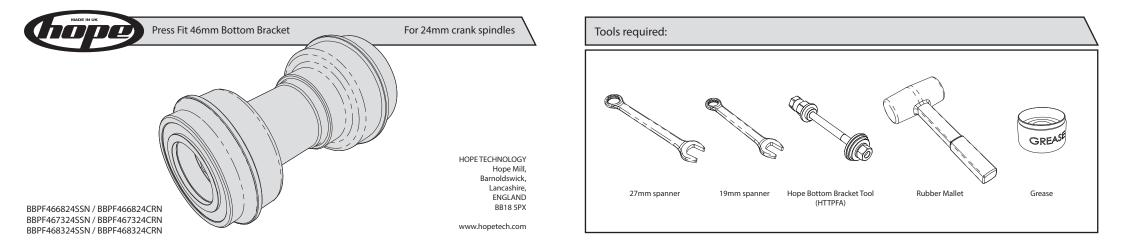
We strongly advise that this bottom bracket is installed and maintained by a competent cycle mechanic, using Hope Bottom Bracket Tool (HTTPFA). This bottom bracket is intended for installation in bottom bracket shells with an internal diameter of 46mm and widths of 68mm, 73mm or 83mm. Check internal edges of bottom bracket shell and remove any burrs or paint build-up prior to fitting.
