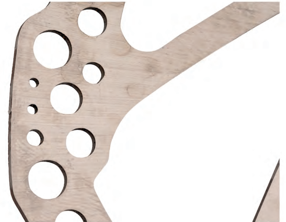
NON BEDDED DISC - GRIND MARKS VISIBLE
